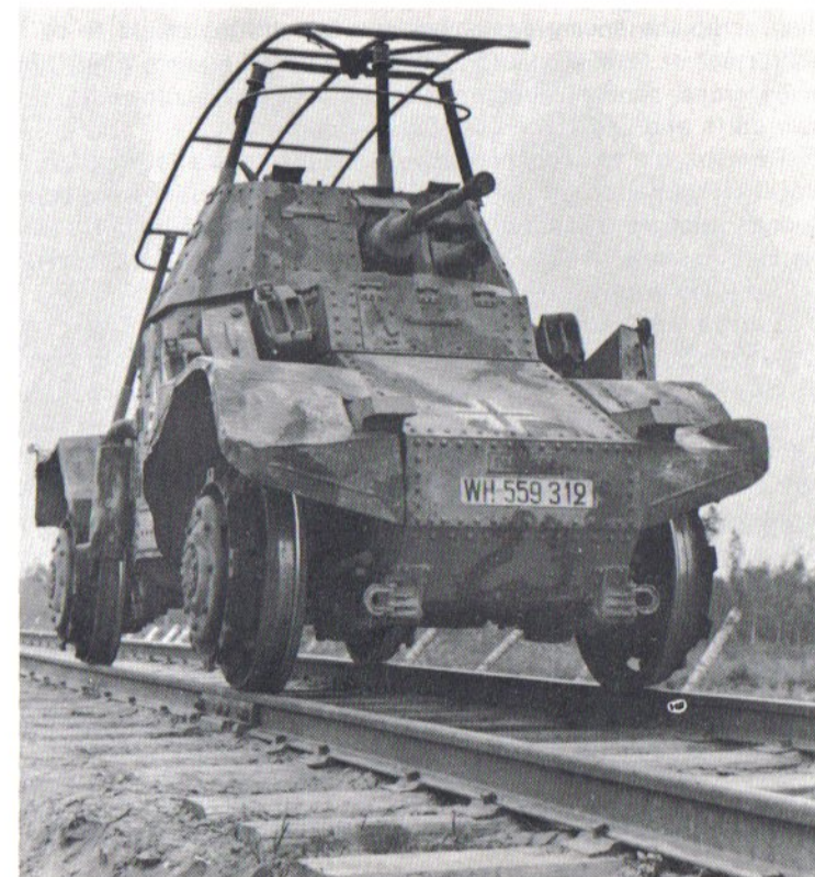
This Panhard 178 is one of 43 of the type that were converted by the Germans into railway protection cars, having their road wheels removed and railroad wheels and axles put in their place. The large frame antenna on the top of the vehicle is another German modification that all of these vehicles had. The French-built 25mm cannon was retained.
