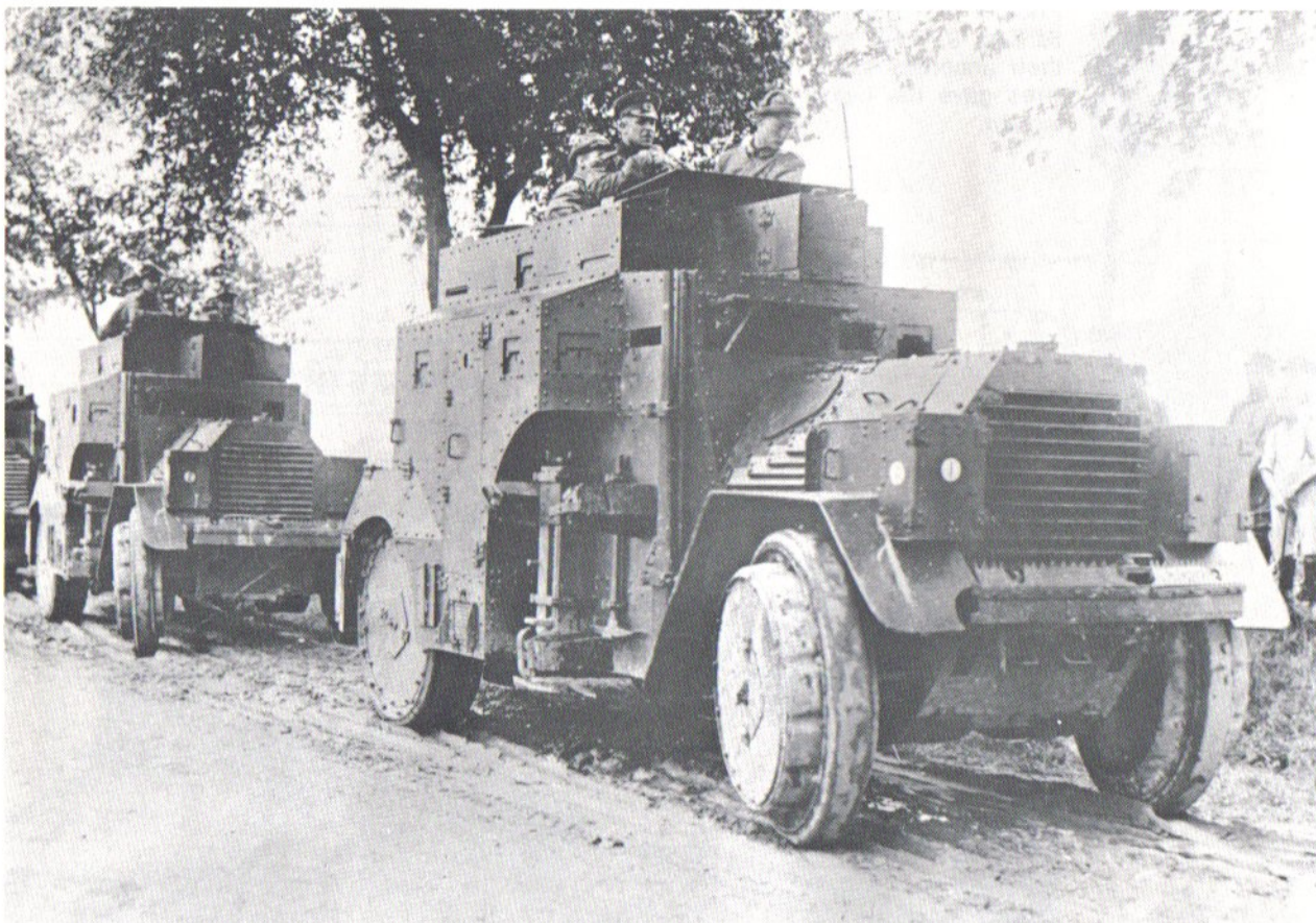
A Krupp-Daimler armored car participating in the Reichswehr autumn maneuvers of 1930 in East Prussia. Although the vehicle is armed with only one machine gun, there were no less than fifteen separate firing ports around the vehicle through which the machine gun could be fired.
