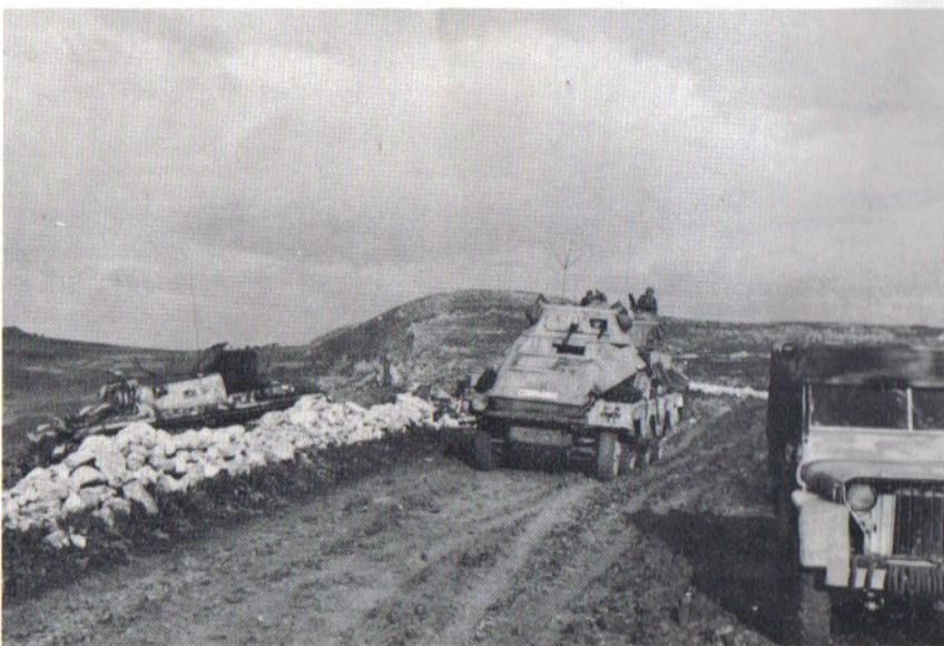
(Above) A good close view of a late model Sd.Kfz. 231 carrying a section of Panzergrenadiers toward an assembly area before a German counter offensive on the Eastern Front. The vehicle in the background is an Sd.Kfz. 233 8-wheeled armored car armed with a short barreled 75mm gun, used for close support.
