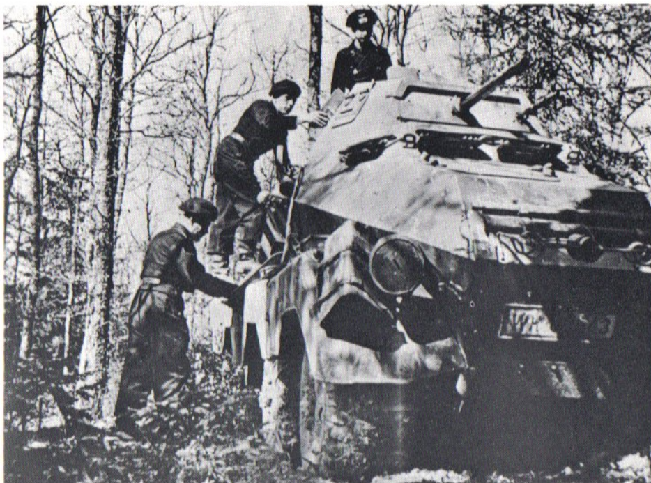
A Wehrmacht armored car crew gets ready to man their Sd.Kfz. 231 'Waffenwagen' during the French campaign of 1940. The crew members are wearing the standard black uniform of the Panzer corps. Note the open visors on the front and sides of the driving compartment.
