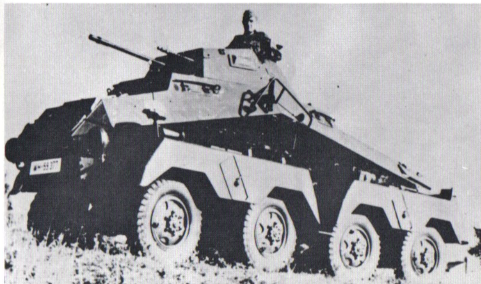
A heavy armored car on the move. These 8-wheeled vehicles had the best cross-country mobility of any of the Wehrmacht's wheeled vehicles, despite their weight of near nine tons. The vehicle's biggest disadvantage was its extremely high silhouette.
