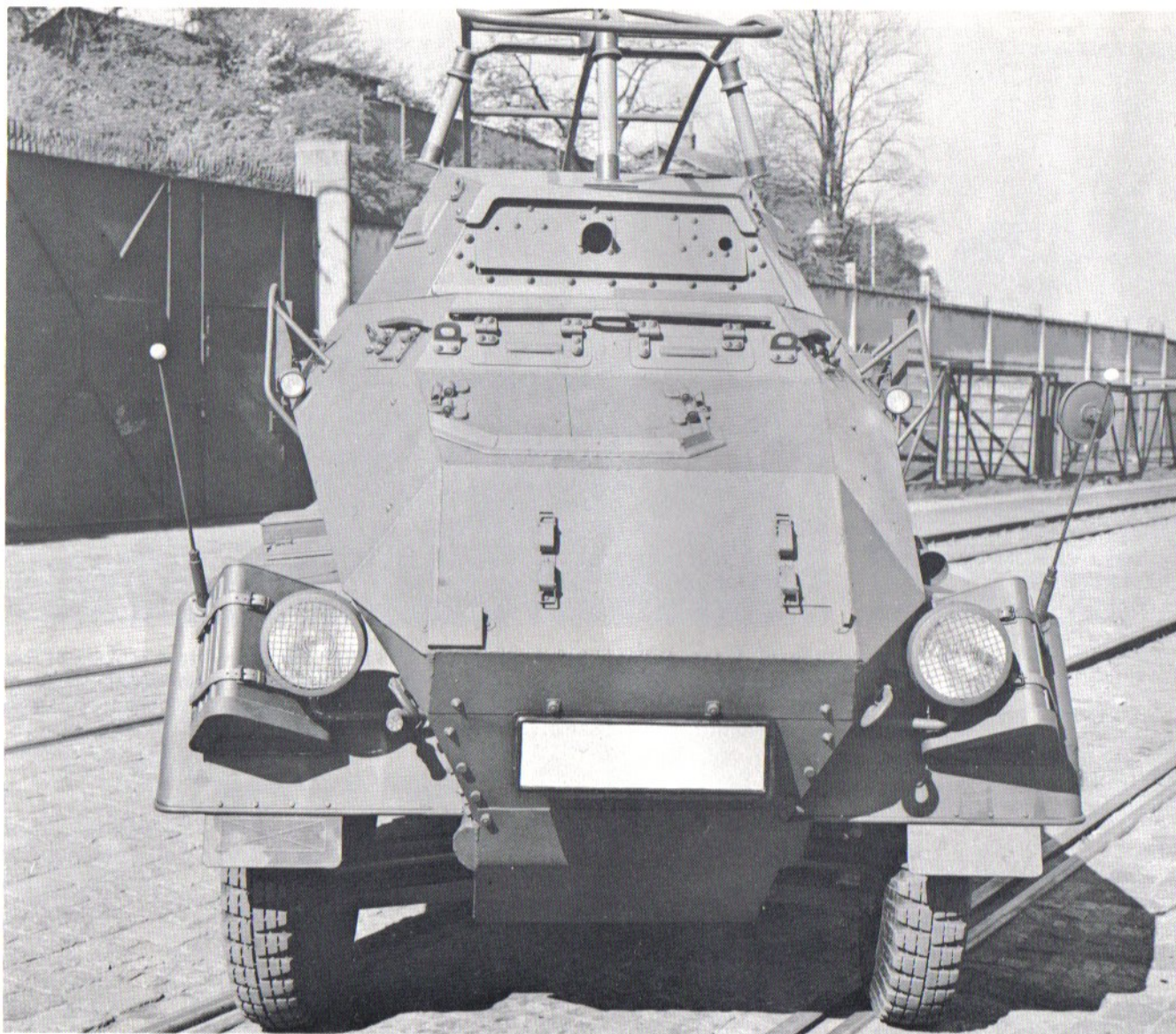
At the Deutsche Werke factory in Kiel, a brand-new Sd.Kfz. 232 waits adjacent to the factory's railroad spur until a train can pick it up for delivery to a Wehrmacht inspection unit. During peak production of these vehicles, the Deutsche Werke factory could turn out up to twenty of these vehicles a day. More could have been produced, but no third, or 'graveyard' shift was worked.
