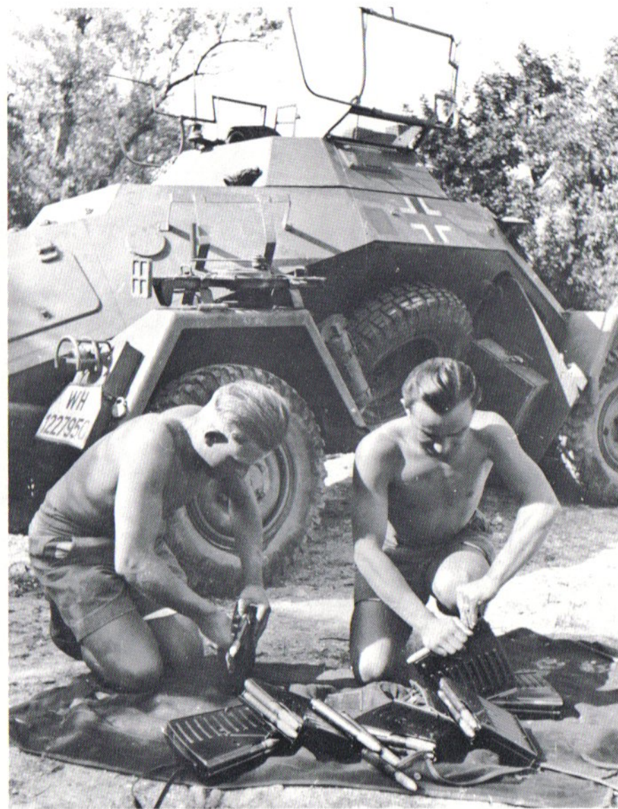
After the armored car's armament has been thoroughly cleaned, two of the crew members begin to prepare the 20mm ammunition magazines which held 10 to 12 20mm projectiles each. Stowage space for 20 magazines was provided in each of these vehicles
