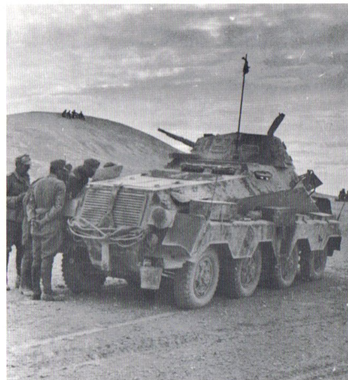
Afrika Korps personnel gather around the engine access hatch of this 8-wheeler to look for any visible signs of damage. Regardless of the precautions taken by Afrika Korps personnel to protect their vehicles from sand, the desert played no favorites.
