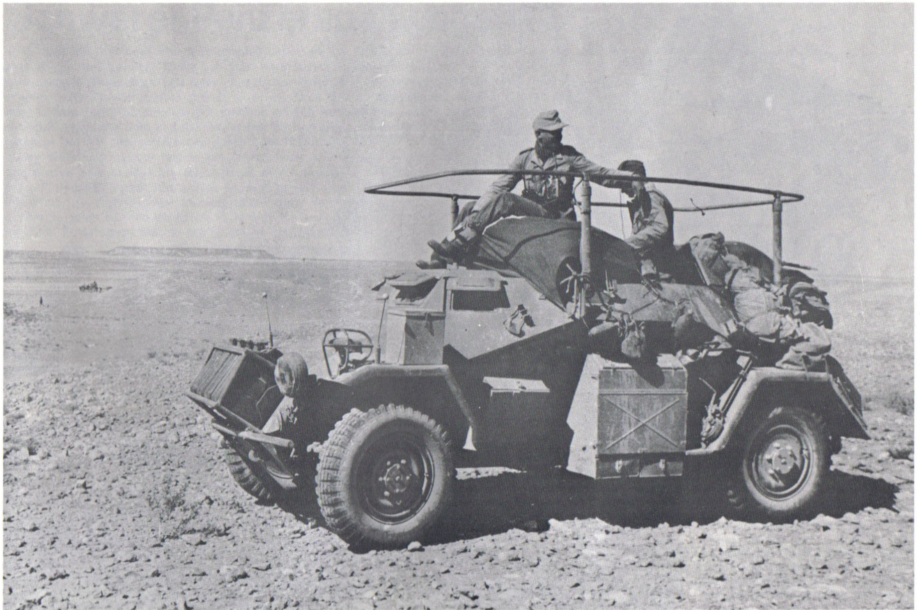
All set for a long range reconnaissance patrol, this Sd.Kfz. 223 features all of the crew's personal gear strapped to the rear decking and at least twenty gallons of spare gasoline in the jerricans on the special rack attached to the front of the vehicle.
