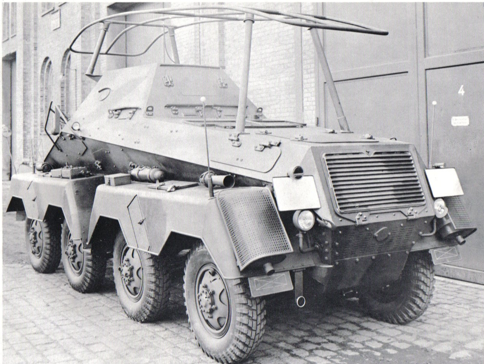
A very nice three-quarter rear view of the newly constructed Sd.Kfz. 263 . This particular vehicle has been camouflaged with a two-toned sand yellow and light brown shadow scheme. A close look will reveal round pistol ports on the sides of the superstructure, two air horns; one facing forward and the other aft.
