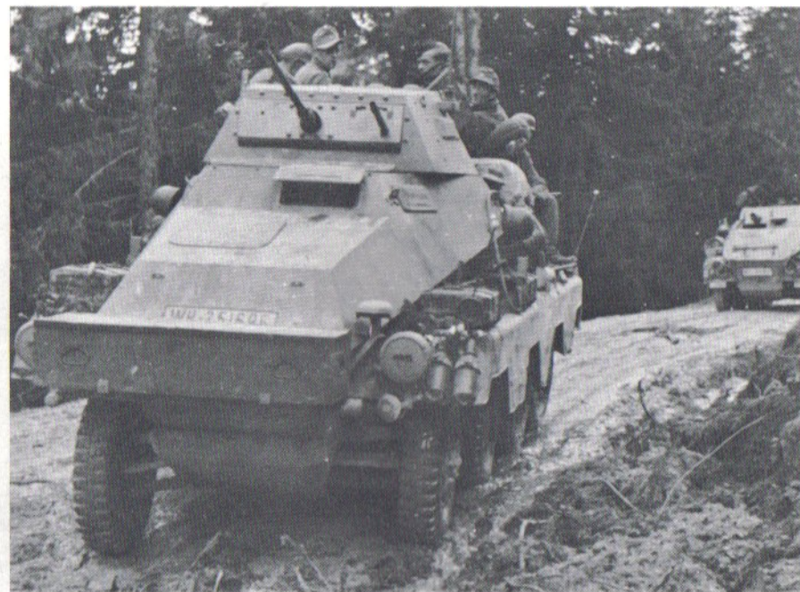
(Above) A good close view of a late model Sd.Kfz. 231 carrying a section of Panzergrenadiers toward an assembly area before a German counter offensive on the Eastern Front. The vehicle in the background is an Sd.Kfz. 233 8-wheeled armored car armed with a short barreled 75mm gun, used for close support.
