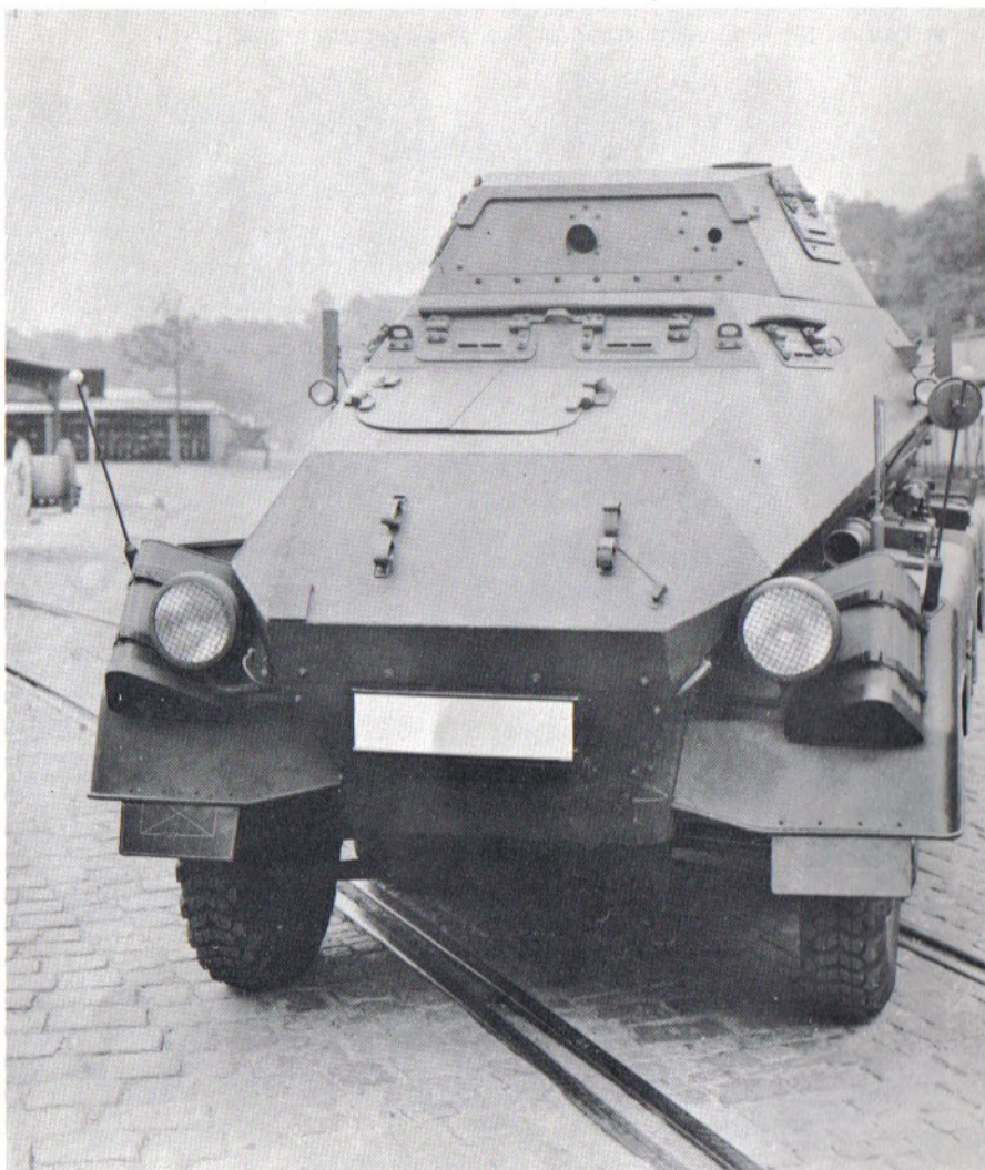
An excellent photograph of a brand-new Sd.Kfz. 231 heavy armored car (' Waffenwagen ') just wheeled out of the Deutsche Werke factory in Kiel. Armament for this vehicle and other equipment was not installed until the vehicles were inspected and accepted by a Wehrmacht or Waffen-SS Ordnance Reception Unit.
