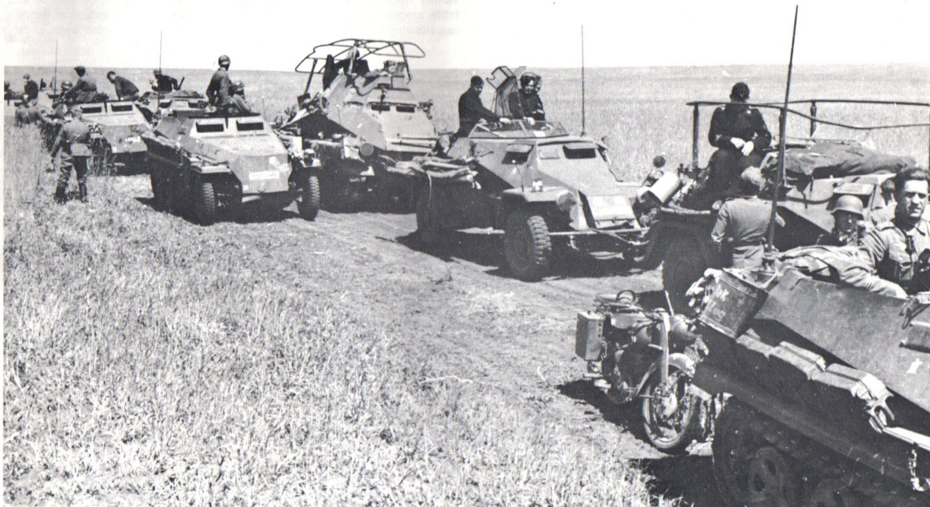
BLITZKRIEG! An armored reconnaissance column of the Grossdeutschland Division pauses during the campaign in the East. Visible in this photo are six separate types of vehicles: five Sd.Kfz. 250 halftracks , one DKW motorcycle , an Sd.Kfz. 223 light armored communications car , two Sd.Kfz. 261 light communications cars (with whip antennas) and an Sd.Kfz. 263 heavy armored communications car .
