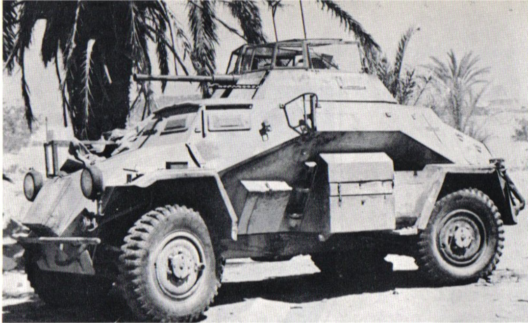
A nice view of an Sd.Kfz. 222 armored car parked next to an oasis during the North African campaign of 1940-1942. The major distinguishing characteristic of this vehicle is its 2cm rapid firing gun and the MG34 machine gun adjacent to it. The vehicle can be further distinguished from the earlier Sd.Kfz. 221 by the obvious 'step' on the rear decking.
