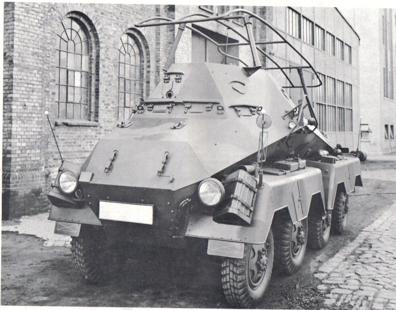
A heavy communications vehicle, Sd.Kfz. 263. Although built along the same lines as its brothers, the Sd.Kfz. 231 and 232, this vehicle had no turret. The superstructure was simply raised in order to accommodate the additional radio equipment necessary for command communications functions.
