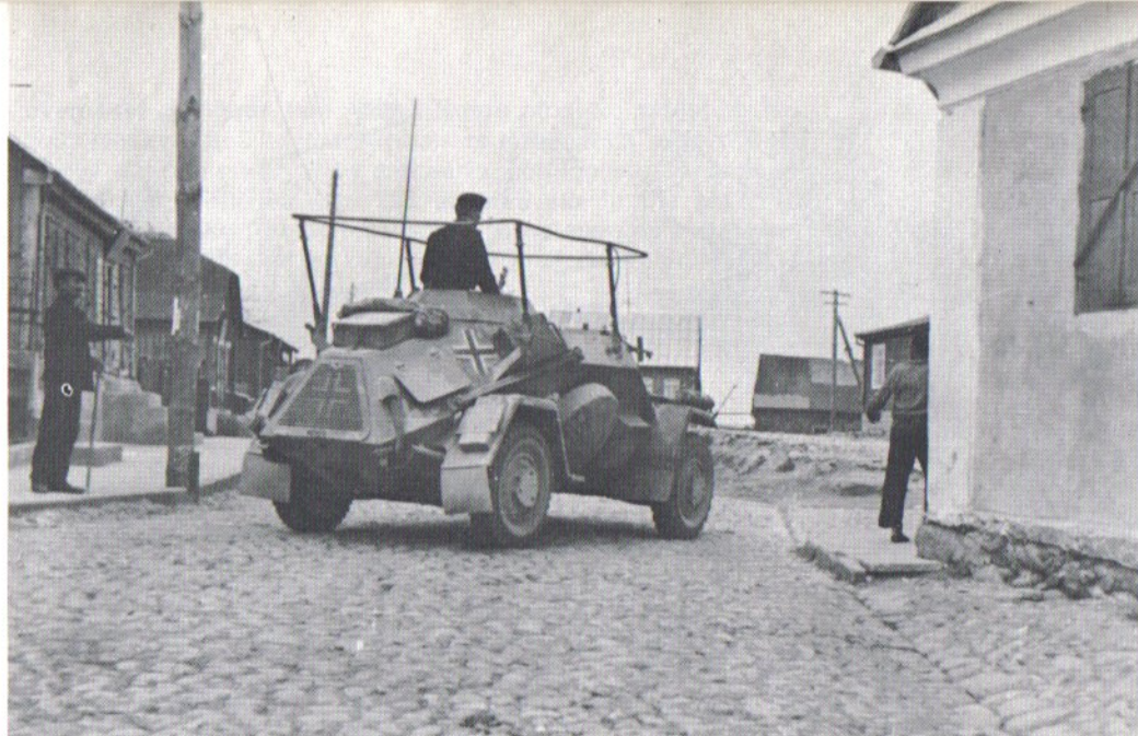
(Left) An Sd.Kfz. 223 radio vehicle with its frame antenna raised rounds a corner in a Greek village as the vehicle commander in the open turret issues directions to his driver. These vehicles had a three-man crew, as did the Sd.Kfz. 222 armored car .
