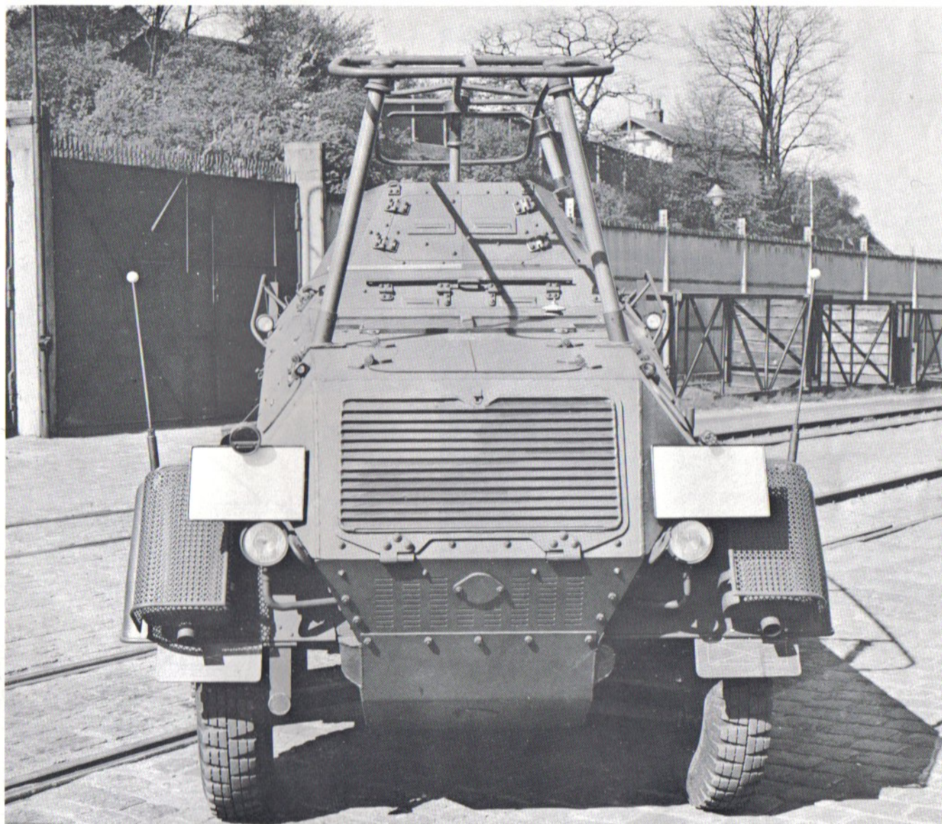
The Sd.Kfz. 232 here differed only from its brother, the Sd.Kfz. 231 by the inclusion of the built-on frame antenna and additional radioequipment. The rods on the fenders with the small white balls at their tops signified the widest part of the vehicle. They enabled the driver to judge distance between obstacles and determine if the vehicle could fit between them.
