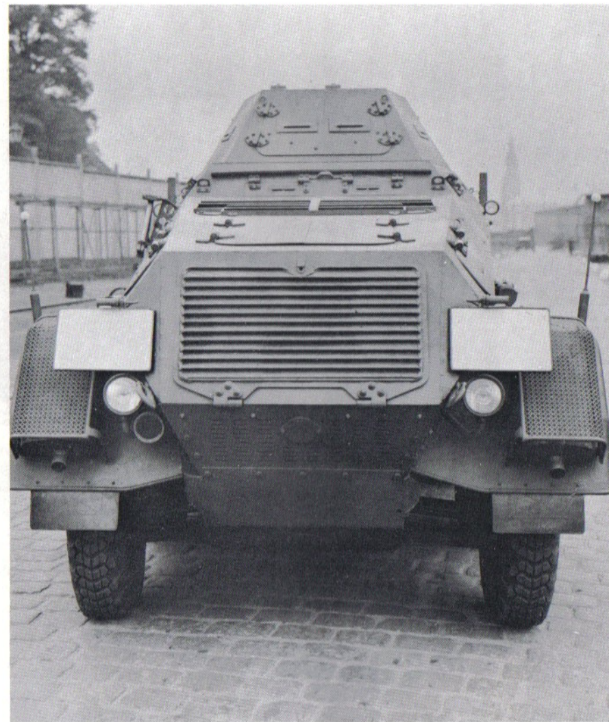
A rear view of the factory-fresh Sd.Kfz. 231 , showing to advantage the alternate set of headlamps just below the license plate holders (still blank) and the rear driver's vision slits just above the air intake grille on the rear top decking.
