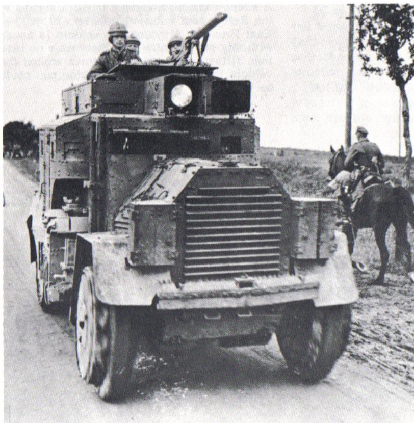
Another view of the big Krupp-Daimler armored car, designated by the Reichswehr as Sd.Kfz. 3 . This shot provides a good view of the searchlight and the headlights in their armored boxes. The extensions, or grouzers, on either side of the solid rubber tires gave the heavy vehicle a bit more buoyancy when moving over soft or muddy terrain.
