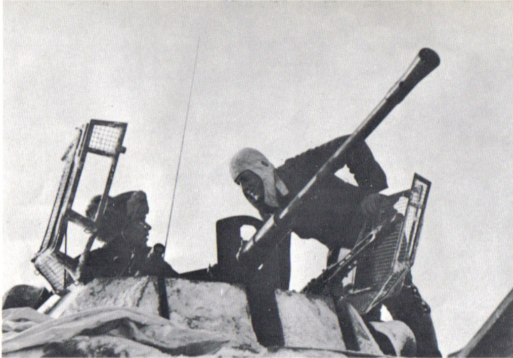
Perimeter watch from the turret of an Sd.Kfz. 222 , January, 1943. Of interest is the MG42 machine gun, instead of its sister, the MG34. The upraised screens on the turret protected the vehicle and crew from grenades or mines thrown into the open turret.
